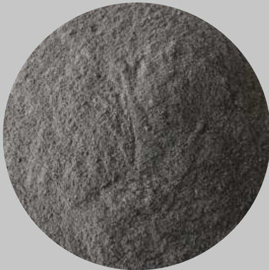
SANDS FOR CONTRUCTION MATERIALS'S CHEMICALS 100-500 mikron. Used in production of ceramic tile adhesives
