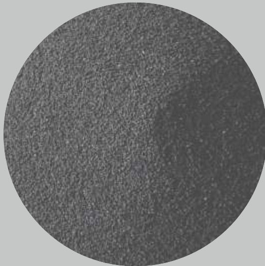
SURFACE HARDENING GRANULES 0,5-2,5 mm. Used for surface hardening purposes
